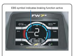
The FW7s EBS has the added advantage of an Electronic Braking System (EBS) for hill descent control.
