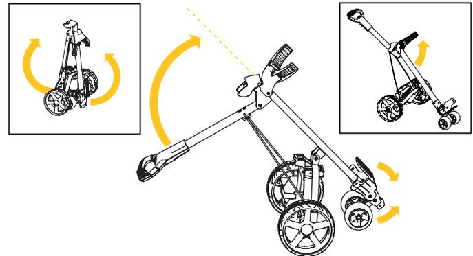
**4** The handle can be set at two heights. Ensure the latch (Fig A.) has sprung into position to lock the handle at the correct height.
