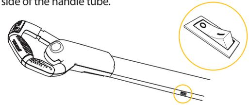
**8** To start the trolley pull back all the way on the handle, the trolley is now ready to go. Move the handle forward to increase the speed of the trolley and pull back to decrease.
