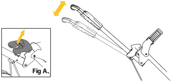
**5** To open the front wheels simply open the bag stay as shown below. The front wheels will automatically move into position.
