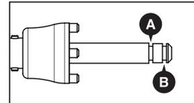
**Groove A.** Wheels will be powered by the motor.
