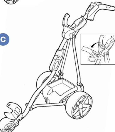
**5** Once charged, connect your battery as shown. The lead acid battery connector is offset so please connect correctly.
