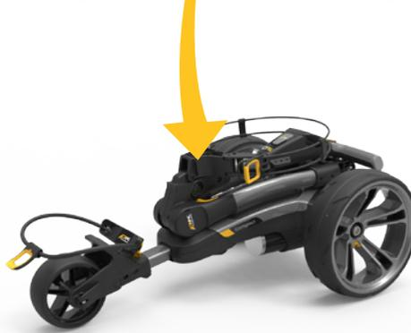
To open the frame, push the yellow front wheel lever towards the bag stay and rotate the front wheel assembly until it locks into place.
