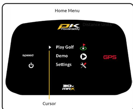
Once your battery is fully charged and connected, your trolley is ready to use. The display will illuminate showing the Home Menu. Rotate the control dial to move the cursor and press to select:
