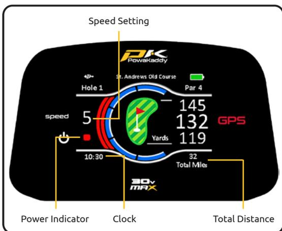
**Clock:** Displays the current time. To adjust the for daylight saving hours, See Section 11.
