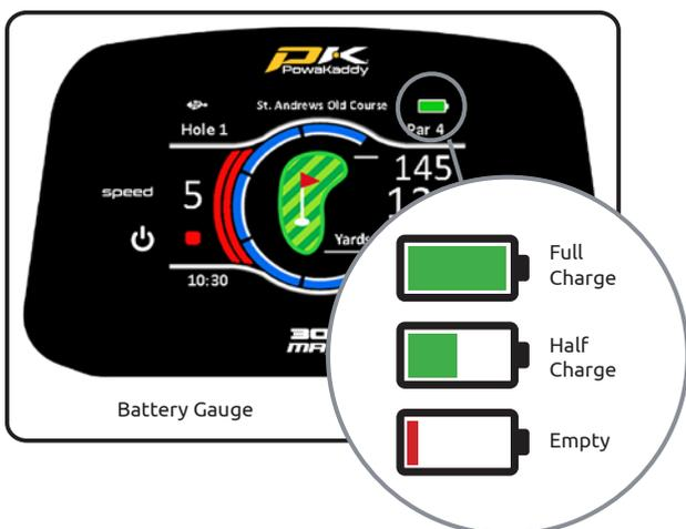
Battery gauge: displayed in the top corner of the display. The charge state of your battery will determine how much of the bar will illuminate.
